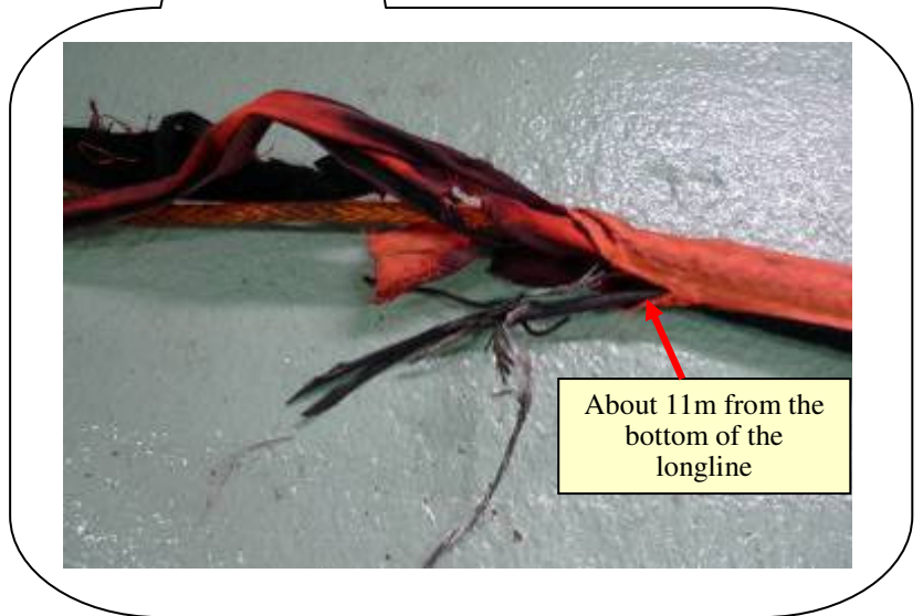
Photo 7 : A closer view of the portion of the damaged longline, about 11 metres from the bottom end
