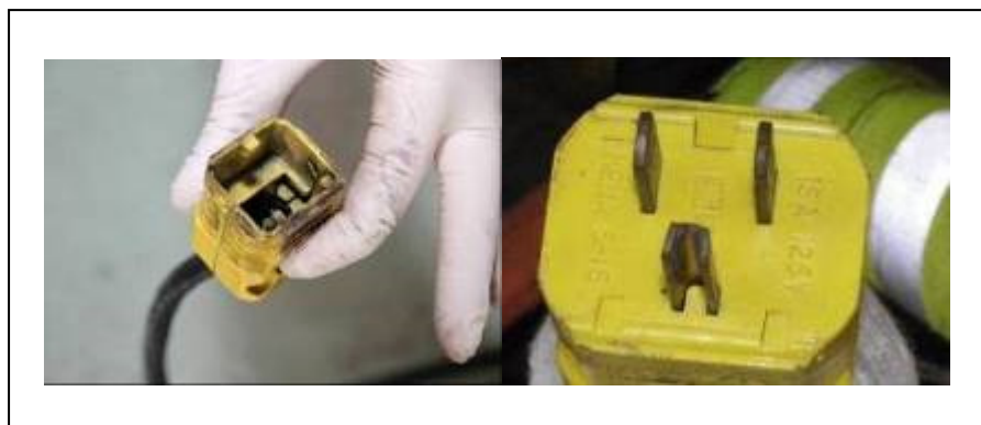
Photo 9 : The damaged electrical plug (left) and example of an undamaged electrical plug (right)
