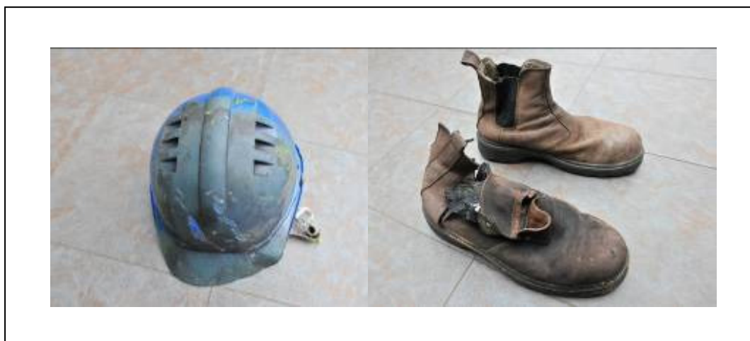
Photo 17 : Burnt PPE of the workers
