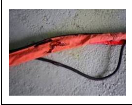
Photo 10 : A close view of the upper portion of the longline where burn marks and slight damage were found
